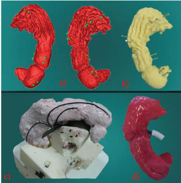
**Figure 2: Silicone stomach fabrication and sensorization: a) virtual position for sensors, b) prototyped mould with screw to locate sensors' position, c) first silicon layer and sensors deposition, d) final stomach model.**
