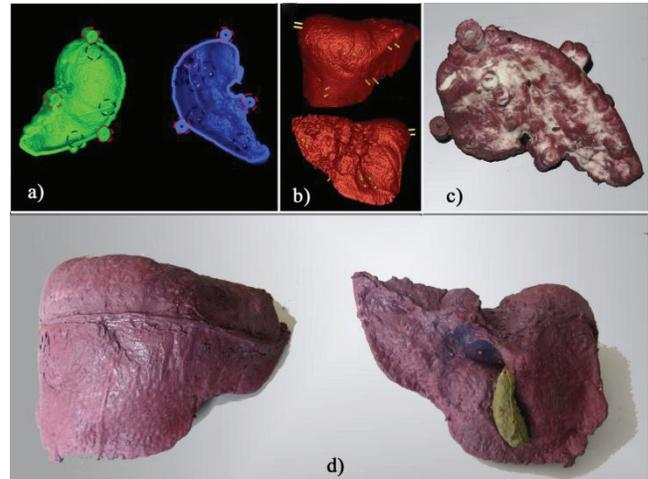
**Figure 3: a) Designed mould for the liver reproduction. In red dotted circles. b) Selected positions for eight Aurora sensor; c) Prototyped mould after silicone injection. d) Final silicone liver front (sx) and back (dx).**
