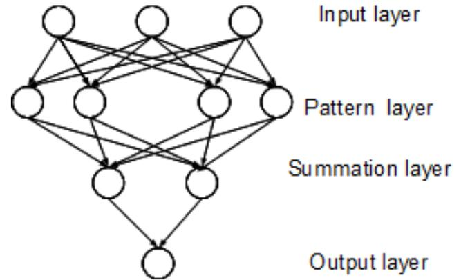
**Figure 4. Probabilistic Neural Network Topology**
