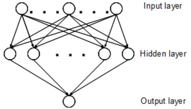
Figure 6. Multi-Layer Perceptron Topology
