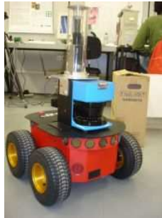
Fig. 4. Robot Pioneer 3-AT used in the experiments.
