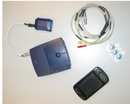
Fig. 1. Epilepsy BAN: electrodes and activity sensor
