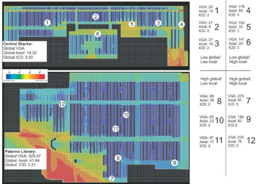
**Fig.2.** The 12 test locations, their global values (left) and local values in space syntax (right).
