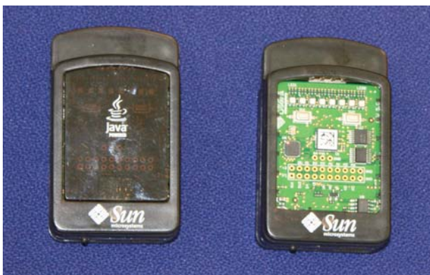
Figure 3: Sun SPOTs as mobile sensor devices
