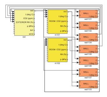
Figure 8. Simulation model of the use-case passive house that was generated semi-automatically by the parser and the semantic engine from passive house floor plan and generic blocks from Bldsimlib library.
