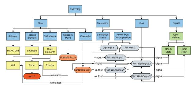
Figure 4. Automation ontology: Machine-understandable knowledge-base formalizing industrial plant, simulation and other engineering knowledge.
