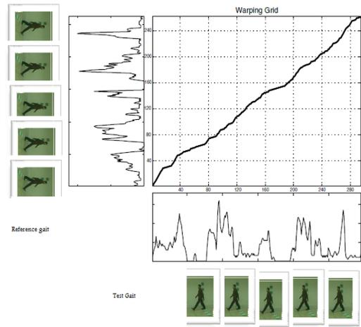
Figure 8. Gait recognition using DTW
