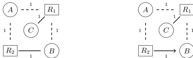
Fig. 1. Left. The SR (and DSR graph) for reaction system (5). Negative edges are depicted as dashed lines, while positive edges are bold lines. This convention will be followed throughout. Right. The DSR graph for reaction system (6), that is, when B is assumed not to affect the rate of the second reaction.
