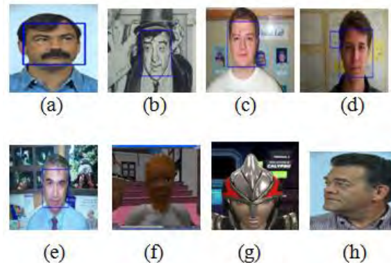
Figure 5: (a) FERET dataset – Positive detection (b) Caltech dataset – Positive sketch detection (c) Caltech dataset – Three background faces detected (d) Caltech dataset – False positive (e) Caltech dataset – False negative, background face at lower right corner (f) Male avatar: Second Life, complex background dataset – Zero detection due to poor illumination (g) Female avatar: Entropia, complex background dataset – Face occlusion (h) FERET dataset: Zero face detection due to 90 degree face rotation to the left.
