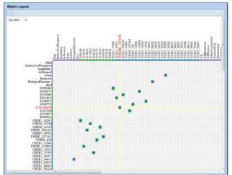
Fig. 2. Mapping Matrix Visualization. Concepts from multiple ontologies are shown as rows and columns. Mappings are shown as colored cells. The user can hover over mappings to highlight row and column. The concepts can be sorted by name or by ontology.
