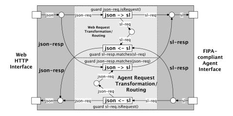
Figure 4. WebGateway architecture for two-way service request handling
