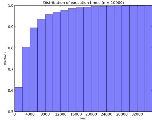
**Figure 5: The cumulative distribution of execution time shows that most of the paths can be found with the lowest execution time ranges.**
