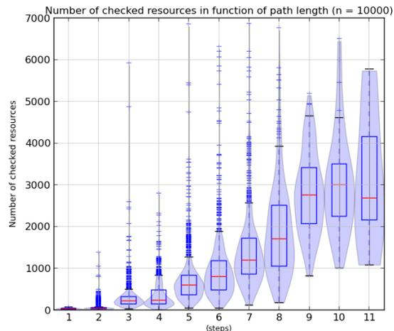
**Figure 7:** The number of checked resources grows exponentially with path length except when the amount of test queries is not high enough to draw a conclusion (path length 10 or 11).
