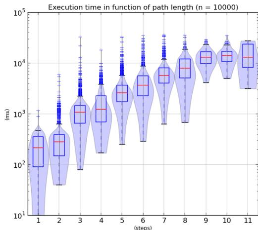
**Figure 6:** The execution time in function of path length appears to be linear in a logarithmic scale.
