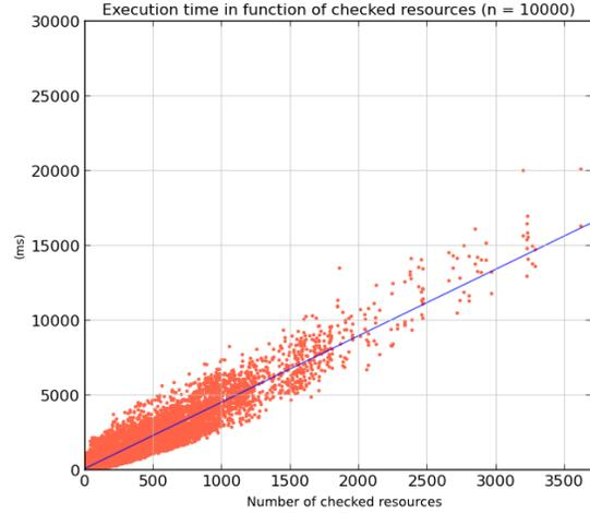
**Figure 4: Execution time ( $y$ ) is approximately a linear function of the checked resources ( $x$ )  $y \approx 4.4x + k$**
