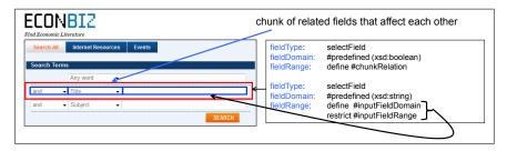
Fig. 3. SDWS field properties (chunk relation)
