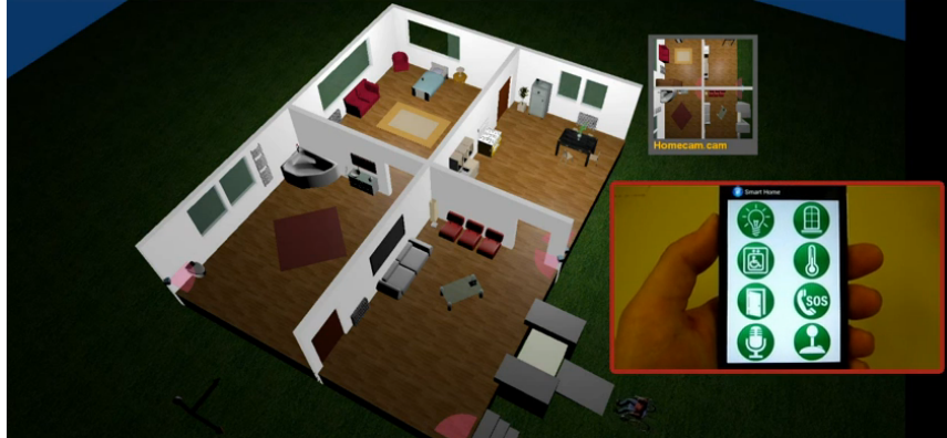
Fig. 1. Virtualized home in Morse: the architecture of the simulation allows to decouple the multi-agent software system controlling the environment from the sensor. Thus, maintaining the same protocols, the intelligent system can be tested in diverse simulators as well as in a real environment.
