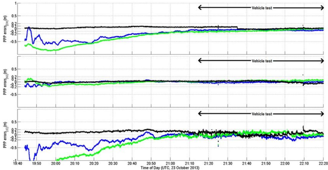
**Figure 5.** Real-time kinematic PPP position (East, North and Up components) errors of the moving vehicle using MADOCA-LEX (blue) and IGS-RT (green) corrections. Post-processed NRCAN PPP solutions (black) are shown for comparison.
