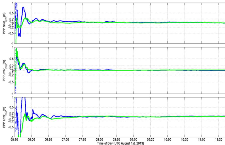
**Figure 4.** Real-time static PPP position (East, North and Up components) errors from using the MADOCA-LEX (blue) and the IGS-RT corrections (green).
