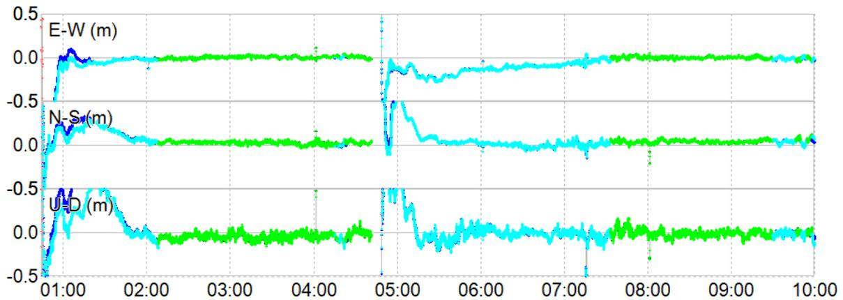
**Figure 7.** PPP-AR solutions calculated using CLK9B based corrections streamed from NTRIP caster (dark green & blue) and from LEX signal (light green and blue). The green points are solutions with fixed ambiguities.
