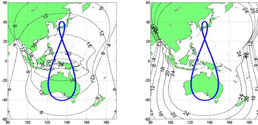
**Figure 3.** Coverage area of QZSS. Left: Number of hours a day QZS-1 satellite is above  $40^\circ$  of elevation. Right: Number of hours a day at least one satellite will be above  $40^\circ$  of elevation once the four satellites constellations are active in 2018.
