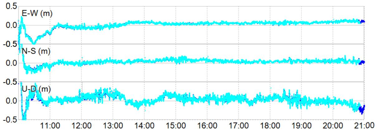
**Figure 6.** PPP solutions calculated using IGS-RT corrections streamed from NTRIP caster (blue) and from LEX signal (cyan).
