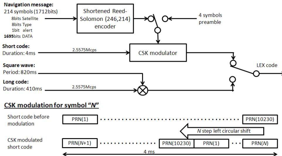
**Figure 1.** LEX signal code modulation (JAXA, 2013).
