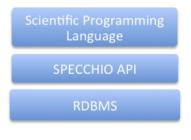
Figure 2: SPECCHIO system layers
