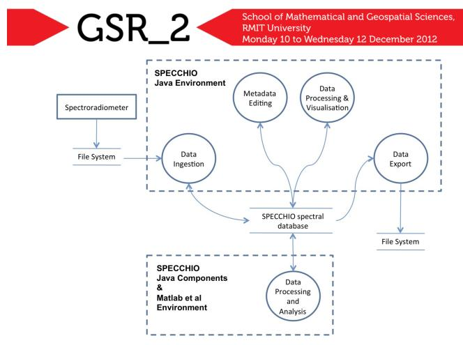
Figure 3: Main dataflows of the SPECCHIO system
