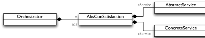
Fig. 5. The modification made to the service composition metamodel from Fig. 2. Note that the remaining classes and feature of Fig. 2 remain the same
