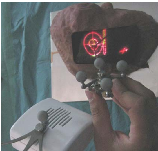
Fig. 3: Projected targeting guidance (with cross hair, alignment circle and depth bar) displayed on the surface of the porcine liver phantom under the tip of the optically tracked ablation needle during the evaluation.
