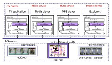
Fig. 2. The architecture of ubiTV
