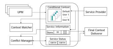
Fig. 13. The architecture of Service Profile Manager
