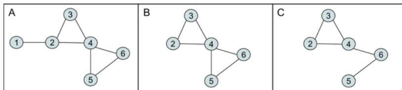
**Figure 1:** Graph B is a *node-induced isomorphism* of Graph A because it is missing a node (1) but preserves all edges between nodes shared in both Graphs A and B. Graph C is a *monomorphism* of A because it is missing a node (1) and an edge (between 4 and 5). Definitions are provided in Section 4.1.
