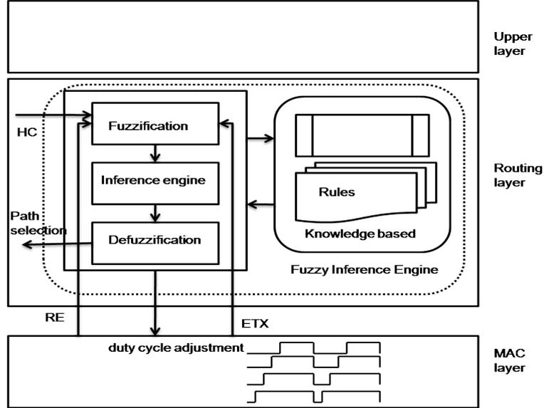
**Fig. 2:** Block Diagram of a proposed approach : IE2MR
