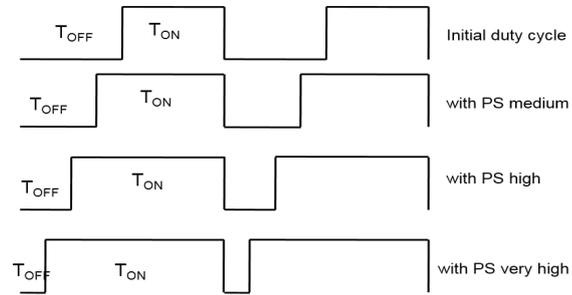
**Fig. 5:** Duty cycle adjustment
