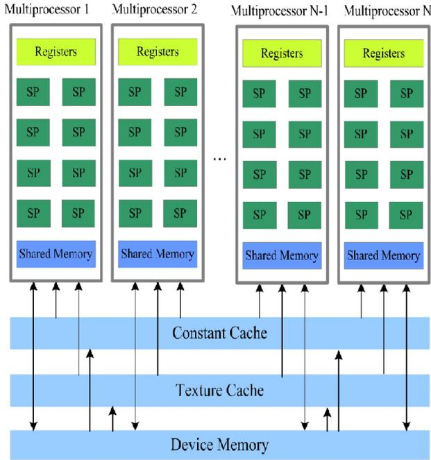
Fig. 2. GPU architecture
