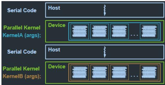
Fig. 2: Model of programming in CUDA
