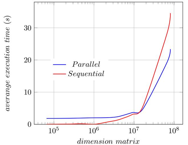
Fig. 6: Comparison between sequential and parallel code on server
