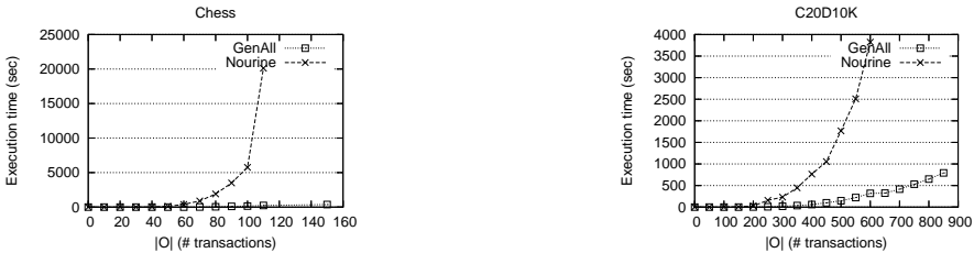
Fig. 5. Execution time of Nourine et al. and GENALL algorithms (case of dense data)
