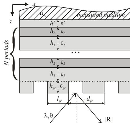
**Fig. 1.** Geometry of the investigated optical sensor consisting of a diffraction grating and a one-dimensional photonic crystal
