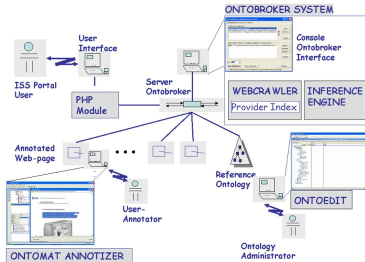
Fig. 4. The software architecture of the semantic portal
