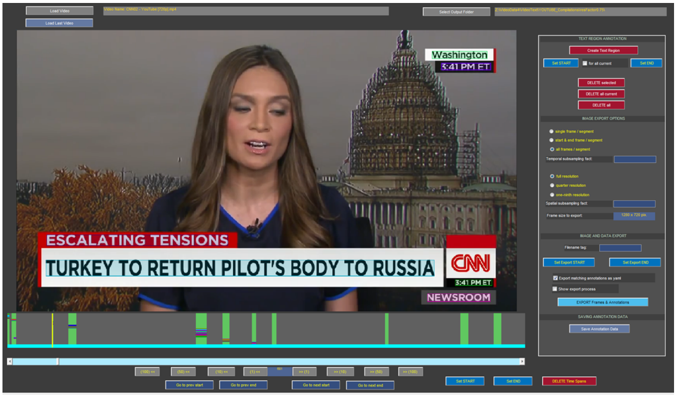
Figure 10. Screenshot of the video annotation tool, capable to quickly annotate large amounts of video text by setting text bounding boxes for selected key-frames and interpolating this information between key-frames.
