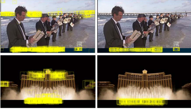
Figure 4. Two difficult (repetitive structures) images demonstrating the classifier accuracy improvement accomplished by using a large synthetic dataset. Yellow rectangles show raw output of the ACF detector trained using real world (a) and synthetic (b) data.
