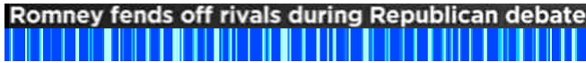
Figure 7. Color-coded confidence distribution (bright = high confidence) for recognizing gaps between characters by learning-based character separation
