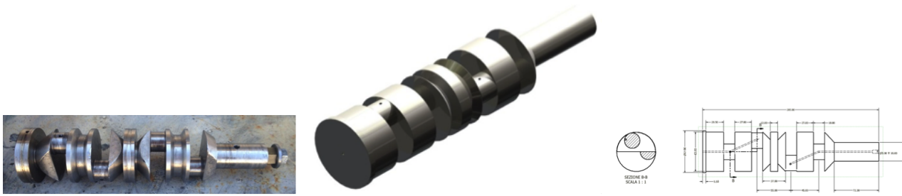
Fig. 5. Camshaft (left) ; 3D model (center); drawing with dimensions (right).
