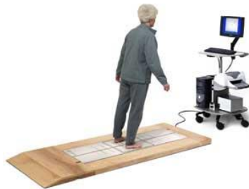
Figure 1. Patient performing a test on a stabilometric platform.
