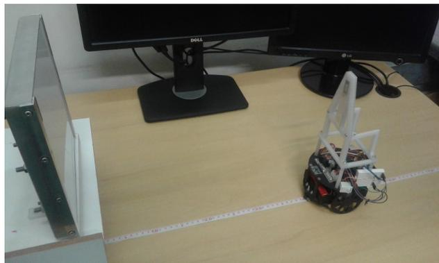
Fig. 13. Implemented mobile robot in front of the reader antenna
