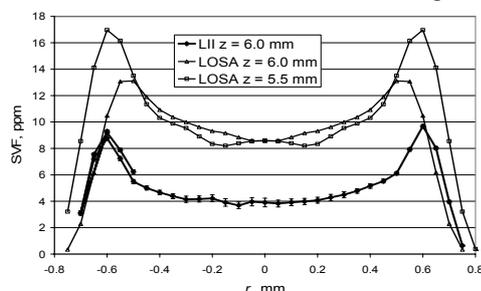
Fig. 1: LII and LOSA SVF,  $p = 1.0$  MPa.
