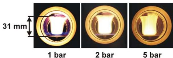
Fig. 1. Premixed ethylene-air flame with an equivalence ratio of  $\phi = 2.1$  at 1, 2 and 5 bar.
