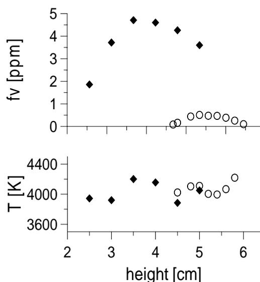
Fig. 1:  $T$  and  $f_v$  axial profile in  $C_2H_4$  (closed diamonds) and  $CH_4$  (open circles) diffusion flames
