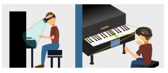
Fig. 1. Illustration of the conceptual design. The user, sitting in front of the piano and wearing an HMD, looks down at the keyboard. When there are notes to be played the respective key is highlighted. Underneath the keyboard there is an image marker which is used for tracking.
