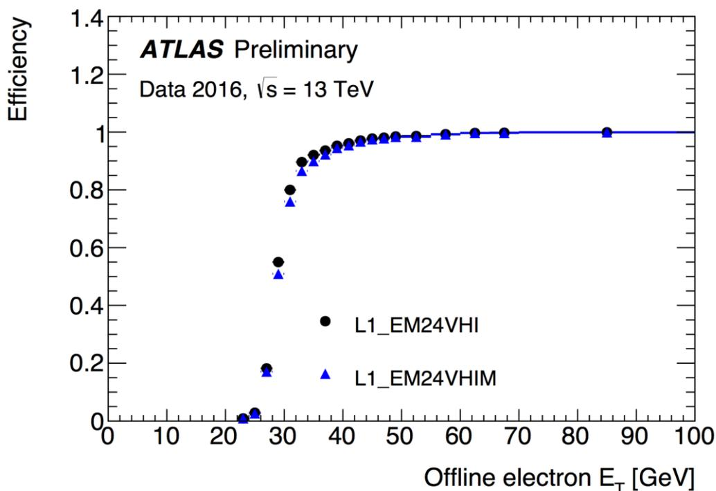
Figure 2. The L1 electron efficiency as a function of offline electron  $E_T$  with a tighter isolation (blue triangles) compared to the previously used looser isolation (black circles). The tighter isolation reduces the trigger rate by 10-15% without significant losses in efficiency [3]
