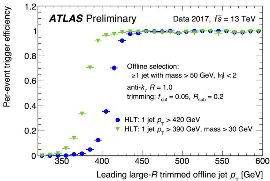
Figure 4. The jet trigger efficiency as a function of offline reconstructed jet  $p_T$  for jets reconstructed using a cone size of  $\Delta R=1.0$ . By adding a requirement on the jet mass to be above 30 GeV (green triangles), it is possible to move the threshold from 420 GeV (blue circles) to 390 GeV without increasing the output rate [6]
