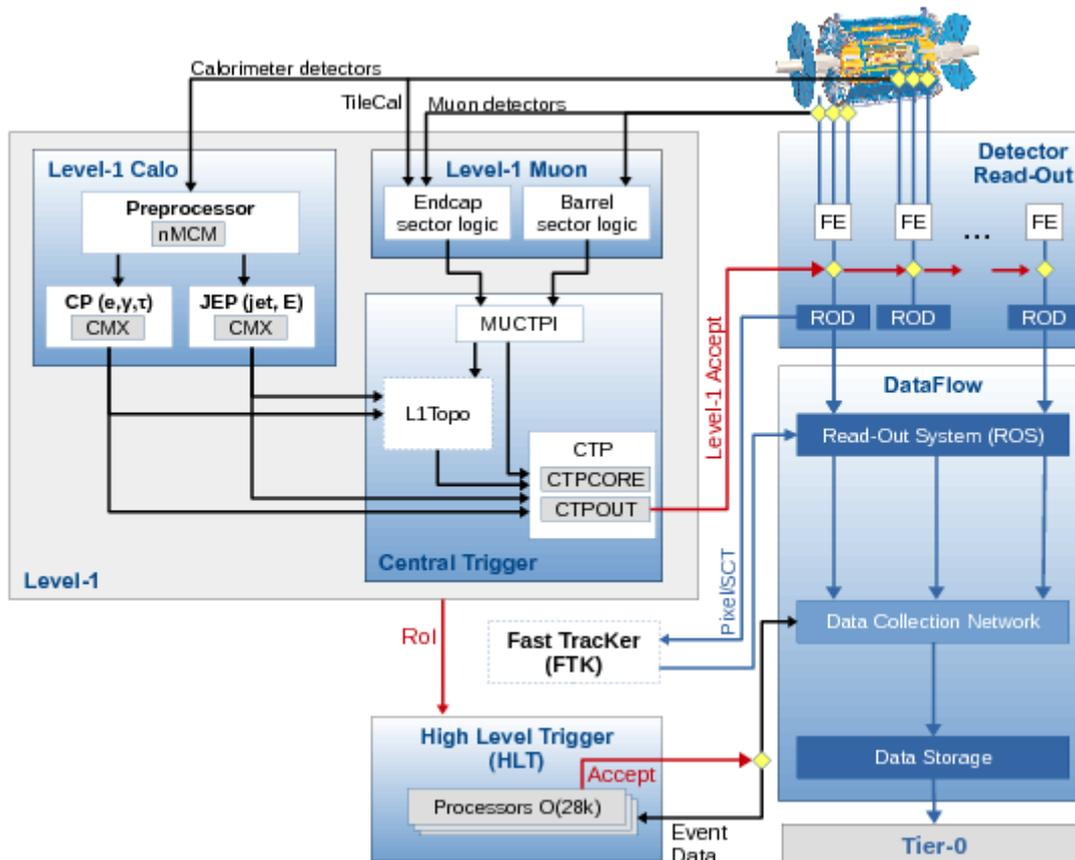
Figure 1. A schematic overview of the ATLAS trigger system consisting of the hardware based L1 trigger, the software based HLT, and the dataflow system
