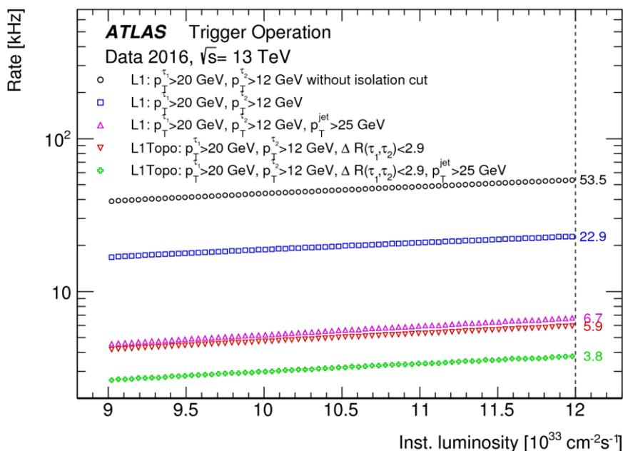
Figure 3. The rates of L1 tau triggers as a function of instantaneous luminosity. The L1Topo triggers including a  $\Delta R$  cut (red triangles and green circles) have a rate of 2-4 times lower than the equivalent triggers without the  $\Delta R$  cut (blue squares and pink triangles respectively) without any loss in efficiency for the physics analysis [4]
