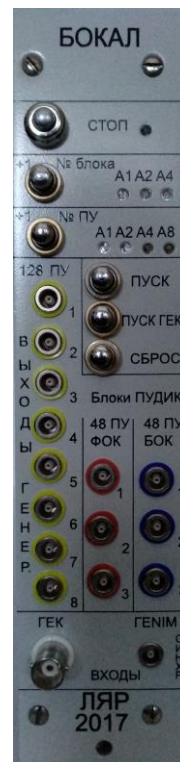
Figure 3. Front view of the module BOKAL (Block for the Organizing of the CALibration)
