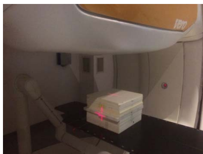
Figure 2: Solid water slabs that used as phantom in the experiment
