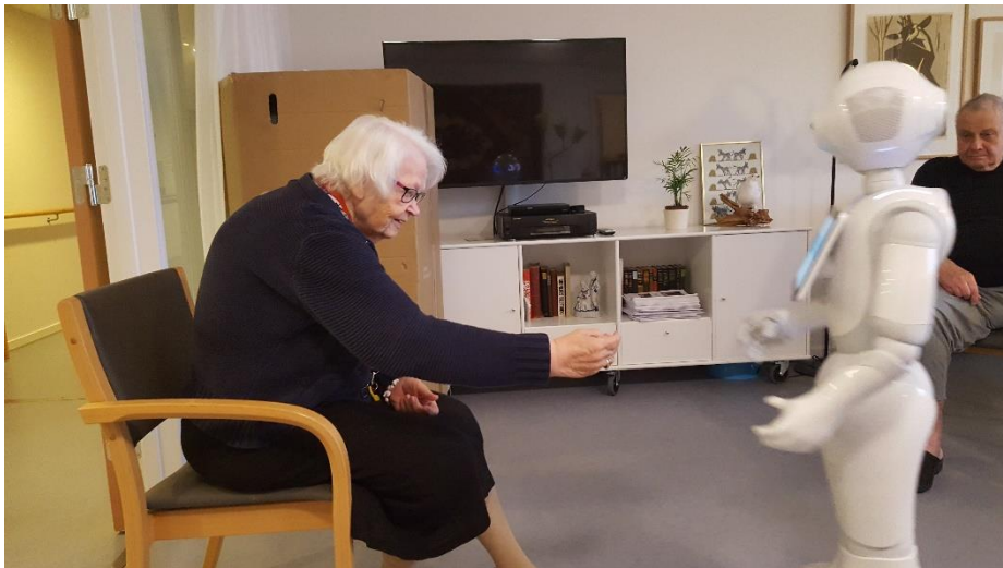
Fig. 5. Robot making animated movements with its arms. The complexity of the movement depends on the player's number of points.
