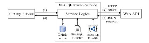
Figure 2: Example implementation of a SPARQL micro-service. A JSON-LD profile interprets the Web API JSON response as a temporary graph G stored in the local RDF triple store. An INSERT query optionally augments G with RDF triples that JSON-LD cannot yield. Lastly, the client's query is evaluated against G.
