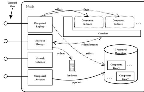
Fig. 1. Logical Node Structure.
