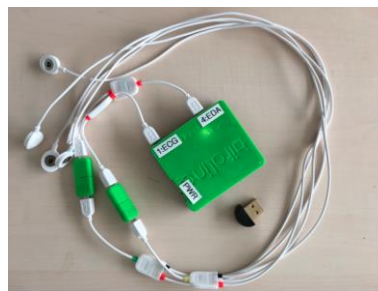
Fig. 2: Bitalino Kit with ECG and EDA sensors plugged in
