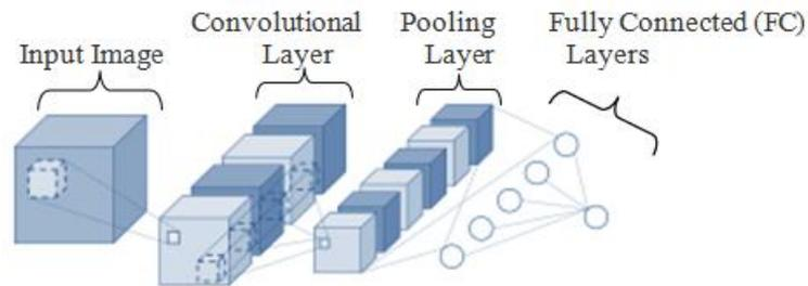
**Fig.1.** An example of CNN architecture.
