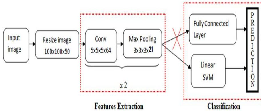
**Fig.1.** The architecture of our model.
