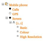
Figure 2: A feature model example (constraints not shown).
