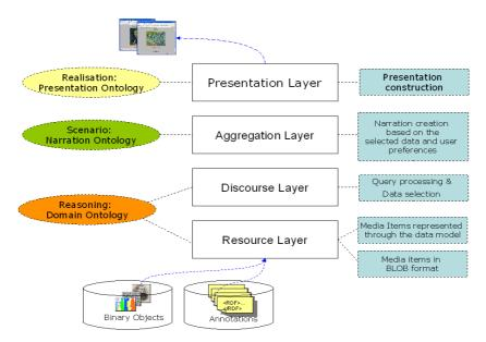
Fig. 4. The layers in the presentation generation architecture
