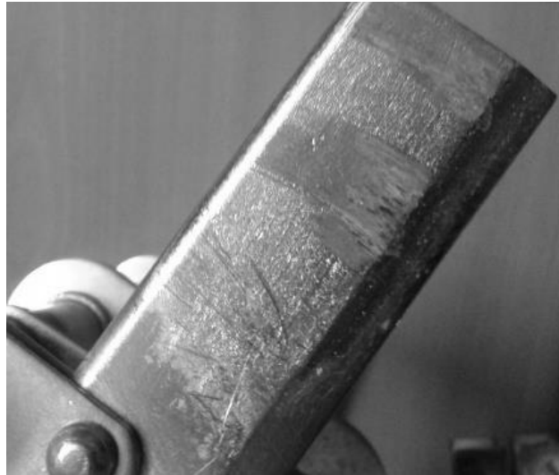
Fig. 3. A metal-coated switch knife after 500 closing/opening cycles
