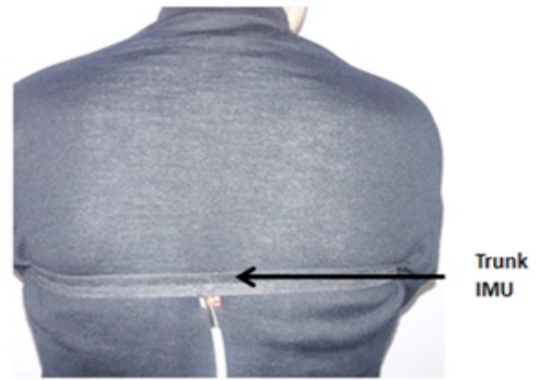
Figure 3- Trunk IMU sensor Placement
