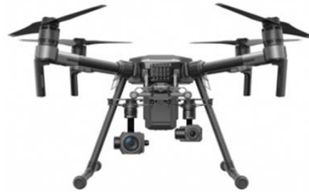
Fig. 2. Drone DJI Matrice 210 with Thermal Imaging Cameras Zenmuse XT and video camera on board [10].
