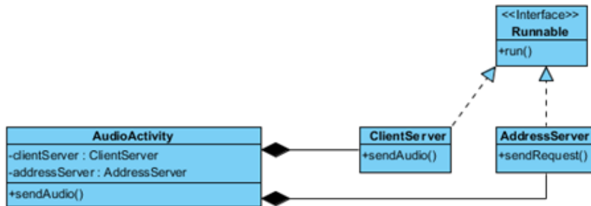
Fig. 2. Class diagram for the server software
