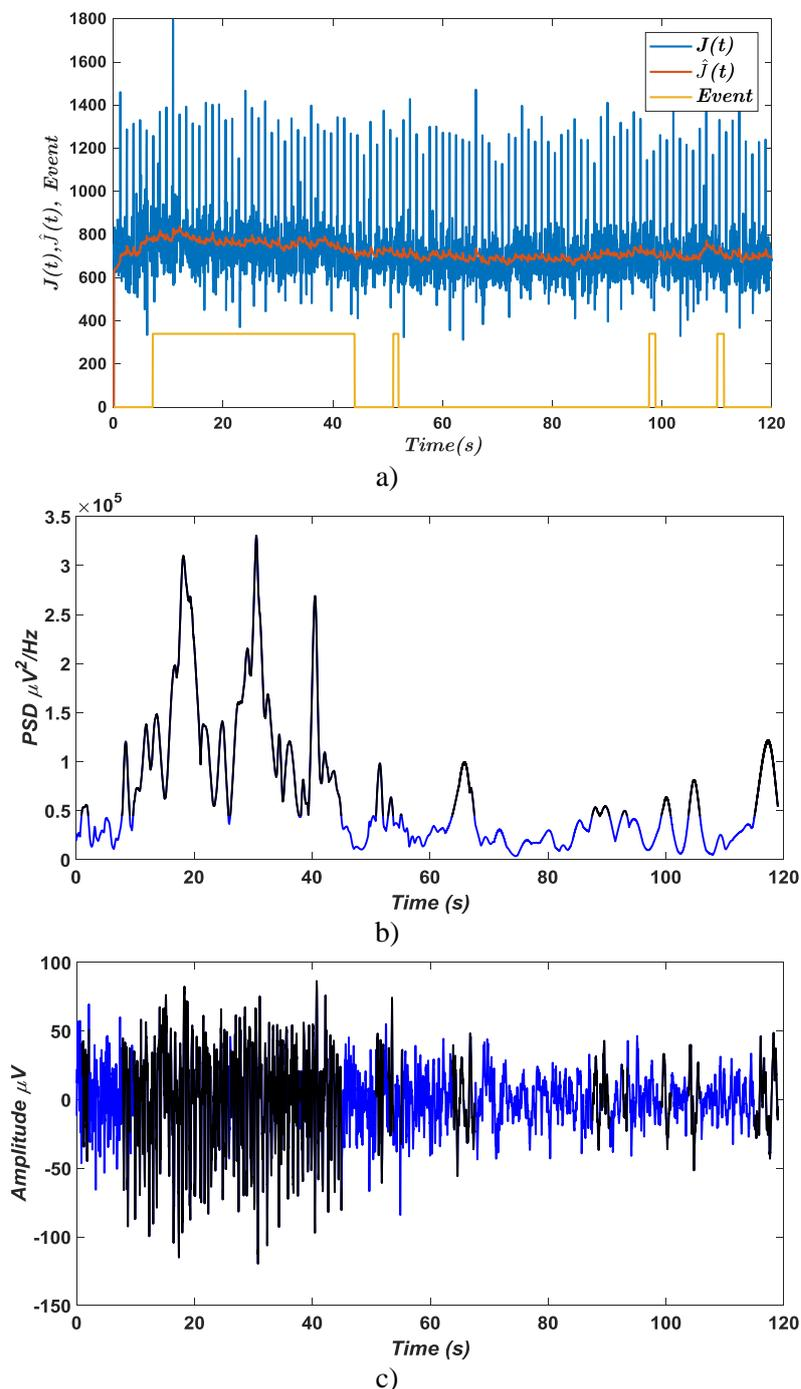
**Figure 4.** Graphs obtained from VEEG monitoring data illustrating detection of non-convulsive seizure: (a) graphs of the criterion  $J(t)$ , estimate  $\hat{J}(t)$ , and event indicator  $Event$ ; (b) projection of the ridge of the wavelet spectrogram on the PSD and time axes; (c) EEG signal in one of the channels, filtered by a Butterworth filter of the 8th order and notch filters.
