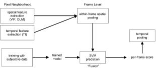
Fig. 1. The scheme of VMAF algorithm.
