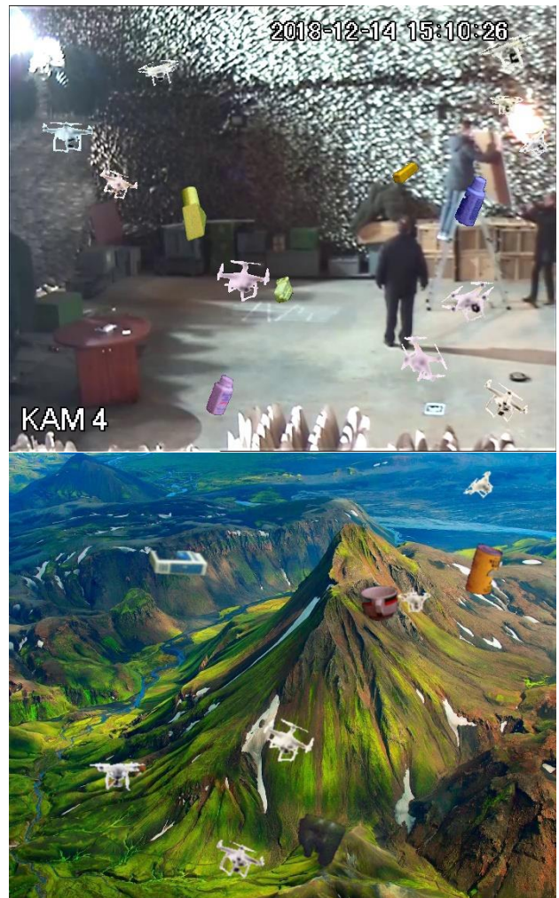
Fig. 5. Examples of training samples. Image having real hangar image as a background and random image.
