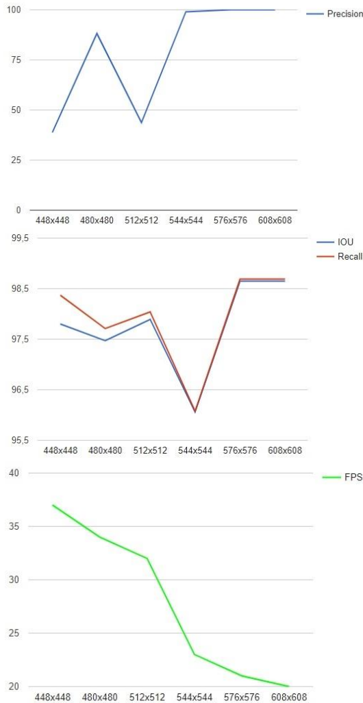
Fig. 3. Dependency of FPS, precision, recall and IoU on image resolution.
